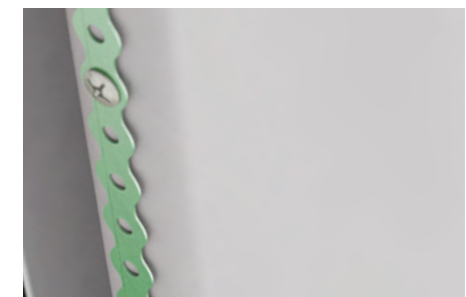
BACK STAPLE COVER STRIP Behavioral Health back upholstery has been altered to allow a staple cover strip to be attached; this will prevent access to the upholstery staples. The cover strip is nylon coated galvanized steel with vinyl coated ends to prevent any sharp edges.
