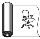
Non-Standard-Cut across the roll "railroad"
