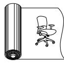
Non-Standard-Cut across the roll "railroad"
