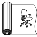
Non-Standard-Cut across the roll "railroad"
