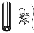
Non-Standard-Cut across the roll "railroad"
