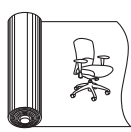
Non-Standard-Cut across the roll "railroad"
